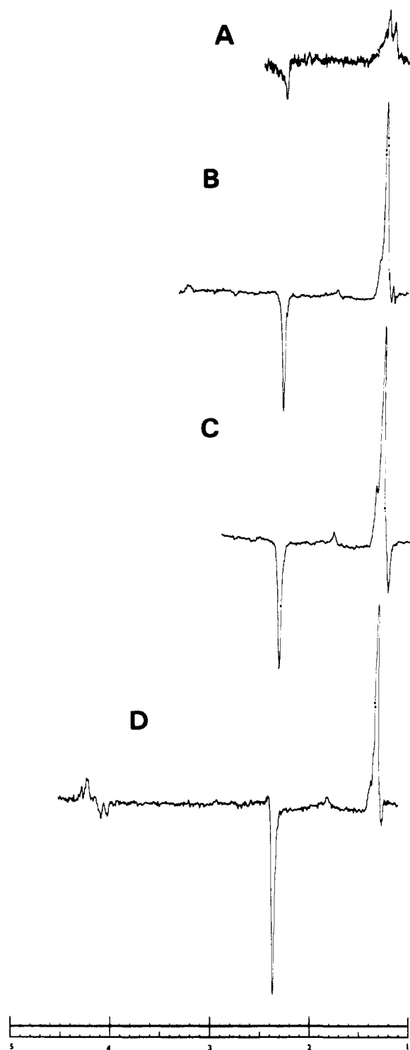
Figure 1. Proton nmr spectra obtained at 100 MHz by mixing a solution containing 0.01 M \text{TiCl}_3 plus 0.1 M \text{H}_2\text{SO}_4 with a solution containing 0.3 M isopropyl alcohol plus 0.1 M \text{H}_2\text{O}_2 . The field increases from left to right: A, mixed outside the probe without the flow system; B, flowing liquid at 40 ml/min; C, flowing liquid at 55 ml/min; D, same as Figure 1B except solvent is changed to \text{D}_2\text{O} .
